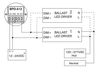
\* DC power can be supplied from the driver with auxiliary DC power output or other source.
