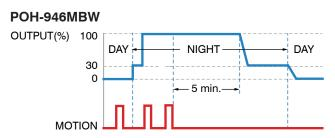
The POH-946MBW will inhibit the LED lighting when ambient light level is higher than 50 lux. If ambient light level is lower than 20 lux, the sensor will automatically dim the LED with 30% power to provide safety night light.
