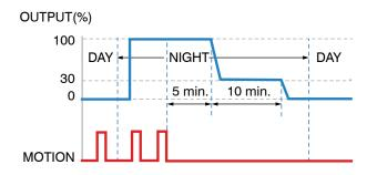
The POM-946MCW will inhibit the associated LED if the ambient light level is higher than 50 lux. If ambient light level goes lower than 20 lux, the sensor will switch on the LED with 100% power when it detects occupancy.
