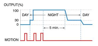
The POM-946MBW will inhibit the associated LED when ambient light level is higher than 50 lux. If ambient light level is lower than 20 lux, the sensor will automatically dim the LED with 30% power to provide safety light level. The sensor will power the LED to 100% when it detects occupancy. The sensor will dim the LED back to 30% if no movement is detected within 5 minutes.
