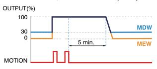
The POM-946MDW will switch on the LED with 100% power whenever it detects occupancy and dim the LED with 30% power if no further movement is detected within 5 minutes.
