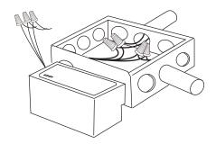
Line voltage wiring connection should be made inside of junction box.
