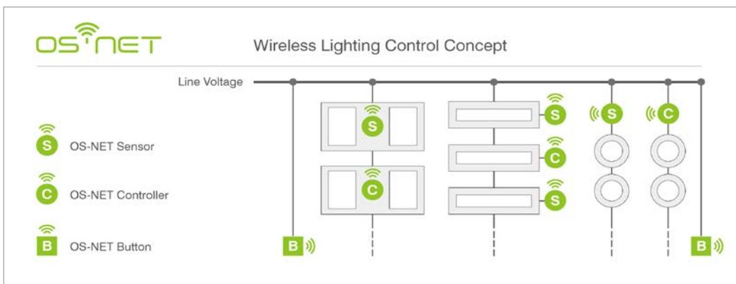
Figure 1. OS-NET Wireless Lighting Control Concept
