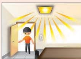
Occupant presence Light auto ON
