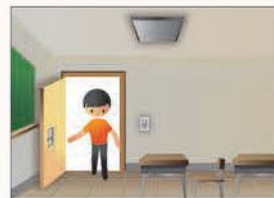
Next occupancy Light remains OFF
