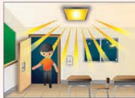
Occupant presence Light auto ON
