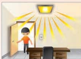
Occupant presence Light auto ON
