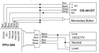
NOTE: Each IR-TEC PPU-300/301 power pack can supply power for up to 3 OS-361DT sensors. When more sensors are connected, multiple power packs may be required.
