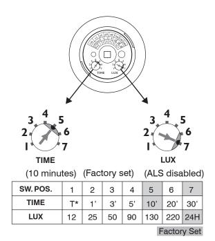
\*T=10 seconds shorten delay for testing convenience. The sensor will automatically resume to the factory default delay setting after 10 minutes, if the potentiometer has not been adjusted to other position.
