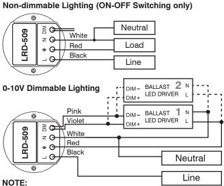
2. Ensure connection of LINE and NEUTRAL are not reversed
