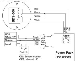
**NOTE:** Each IR-TEC PPU-300/301 power pack can supply power for up to 3 BDS-600SS sensors. When more sensors are connected, multiple power packs may be required.
