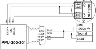
NOTE: Each IR-TEC PPU-300/301 power pack can supply power for up to 6 BOS-515 sensors. When more sensors are connected, multiple power packs may be required.
