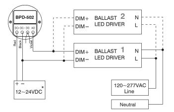
\* DC power can be supplied from the driver with auxiliary DC power output or other source.
