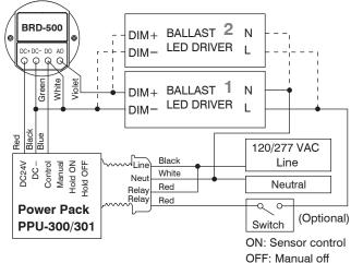
NOTE: Each IR-TEC PPU-300/301 power pack can supply power for up to 6 BRD-500 sensors. When more sensors are connected, multiple power packs may be required.
