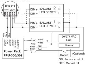
NOTE: Each IR-TEC PPU-300/301 power pack can supply power for up to 6 BRD-510 sensors. When more sensors are connected, multiple power packs may be required.
