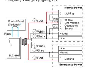
4. Low Voltage Sensor with Power Pack Control of Normal and Emergency Lighting
