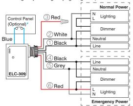
Line Voltage Sensor Control of Normal and Emergency Lighting Normal: Sensor control ON/OFF switching Emergency: Emergency lighting ON
