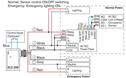
2. Line Voltage Sensor Control of Normal and Emergency Lighting with Dimmable Lighting
