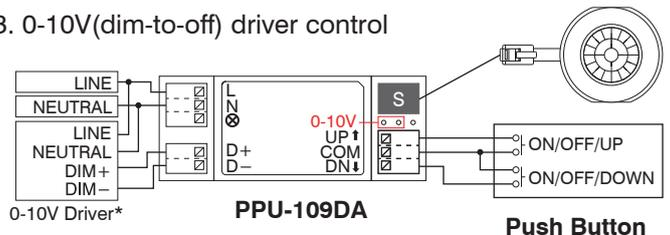
\*Note: for the driver that cannot turn off the light at 0V, please try wiring diagram 2 above.
