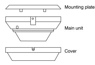
Connect the wires according to the wiring diagram of the desired control mode. Replace the main unit, then test can be conducted.
