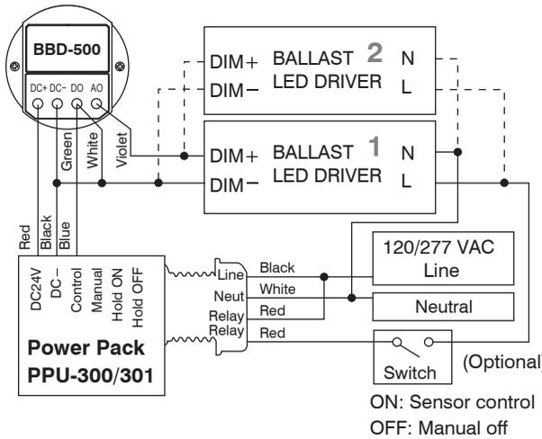
**NOTE:** Each IR-TEC PPU-300/301 power pack can supply power for up to 4 BBD-500 sensors. When more sensors are connected, multiple power packs may be required.
