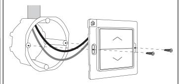
NOTE: Do NOT mount the device upside down. NOTE: Ensure to place the device at least at 1.5m (5 ft.) away from any Wi-Fi router as they can mask or delay signals.
