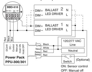
NOTE: Each IR-TEC PPU-300/301 power pack can supply power for up to 4 BBD-510 sensors. When more sensors are connected, multiple power packs may be required.
