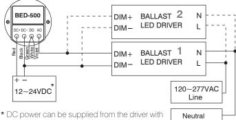
\* DC power can be supplied from the driver with auxiliary DC power output or other source.
