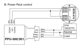
NOTE: Each IR-TEC PPU-300/301 power pack can supply power for up to 6 BOS-515 sensors. When more sensors are connected, multiple power packs may be required.
