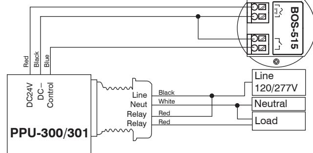
NOTE: Each IR-TEC PPU-300/301 power pack can supply power for up to 6 BOS-515 sensors. When more sensors are connected, multiple power packs may be required.
