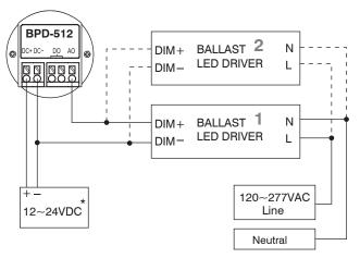
\* DC power can be supplied from the driver with auxiliary DC power output or other source.
