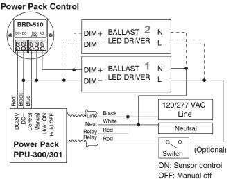
NOTE: Each IR-TEC PPU-300/301 power pack can supply power for up to 6 BRD-510 sensors. When more sensors are connected, multiple power packs may be required.
