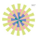
Mounting Height2.4m3.0m3.6m4.2mCoverage (dia.)6m7.5m9m10.5m
