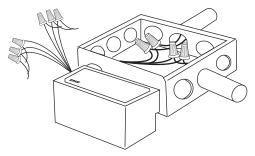
Line voltage wiring connection should be made inside of junction box.
