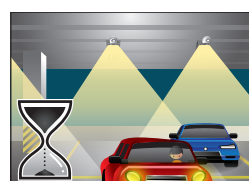
Occupant leave - Delay time start Light remains at HIGH DIM/ SmartDIM**
