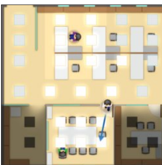
People leave the space, Local lights down to LD after delay elapsed.
