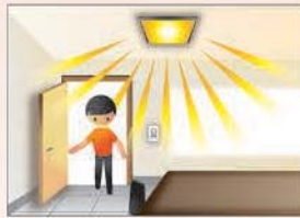
Occupant presence Light auto ON
