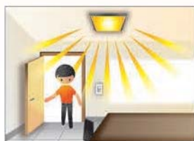
Next occupancy Light auto ON
