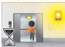
Occupant leave – Delay time start Pole 2 Light remains ON
