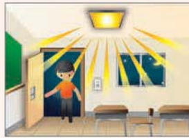
Occupant presence Light auto ON
