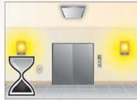
Delay time end – 5 minutes start Pole 1 Light auto OFF Pole 2 Light remains ON
