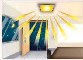
Occupant presence Light auto ON
