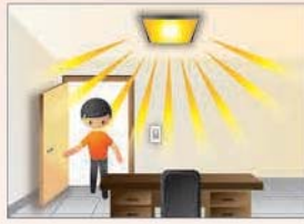
Occupant presence Light auto ON
