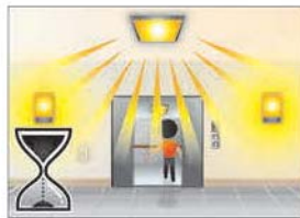
Occupant leave – Delay time start Pole 1 Light remains ON Pole 2 Light remains ON
