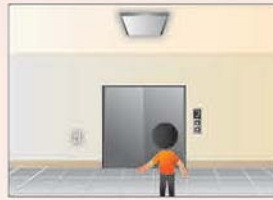
Occupant presence Light remains OFF
