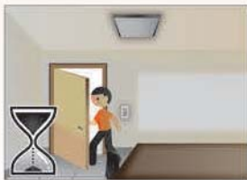
Occupant leave – Delay time start Light remains OFF
