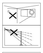
Do not install where the detector is in or facing direct or reflected sunlight, windows onto main roads (car head lights).
