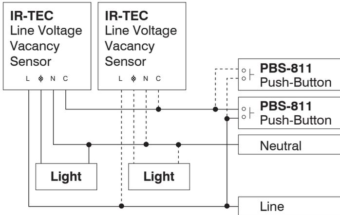
NOTE: The button should provide same phased AC mains power-through momentary contact.
